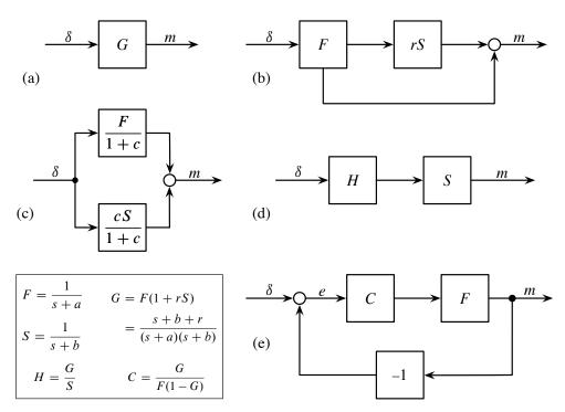
**Figure 2.** Alternative models that yield identical biexponential decay. The text describes each panel. The parameters can be matched to the generic model in Equation (1). with r = c(a - b)/(1 + c).
